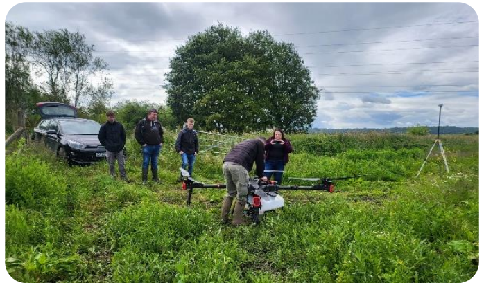
XAG P100 Pro agricultural drone used to apply Typha seed in a gel suspension
